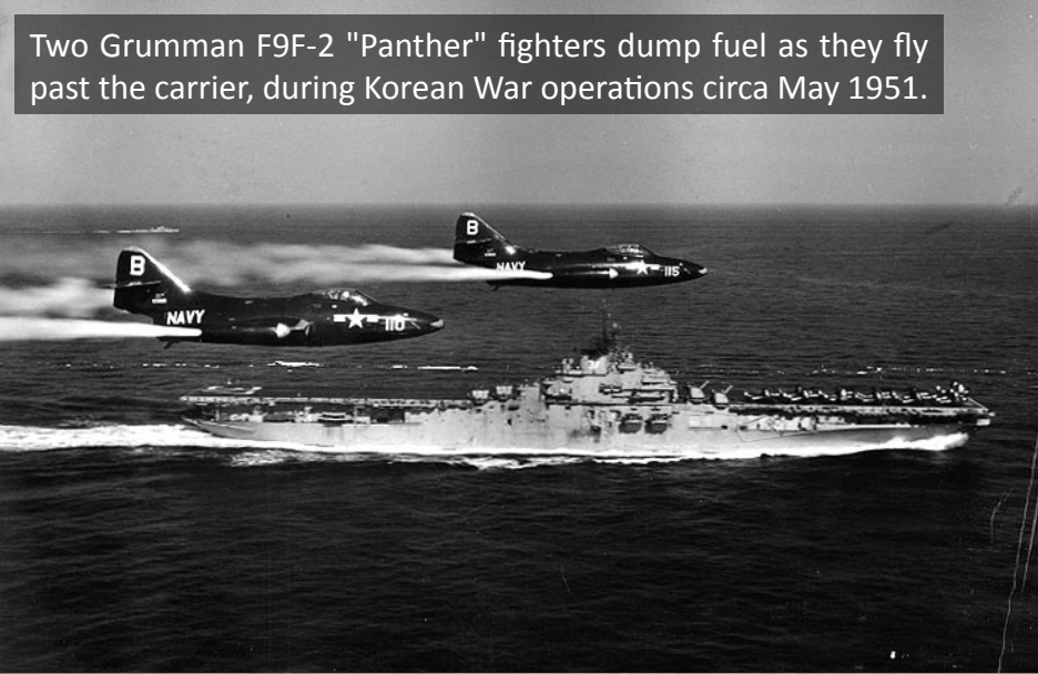
Two Grumman F9F-2 "Panther" fighters dump fuel as they fly past the carrier, during Korean War operations circa May 1951.
